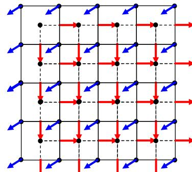
$$\frac{\partial}{\partial t} \mu H_x(\underline{\mathbf{R}}, t) = \frac{\partial E_y(\underline{\mathbf{R}}, t)}{\partial z} - J_{mx}(\underline{\mathbf{R}}, t)$$
